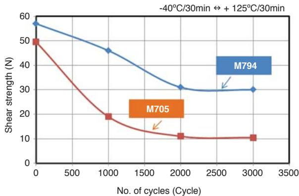
Fig. 9: Comparison of thermal fatigue resistance of alloys
