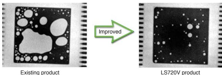
Fig. 6: LS720V flux reduces the generation of voids.
