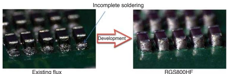
Fig. 3: Melting condition of Type 6 powder under the same condition
