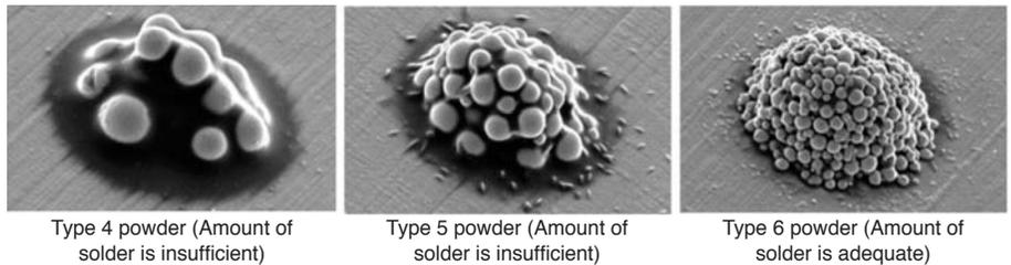
Fig. 2: Solders are printed using a pattern with an aperture of 130μmφ and mask thickness of 60μm.
