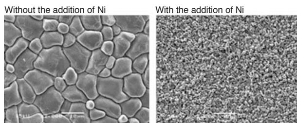
Fig. 7: Comparison of IMS alloy structure after subjected to a reflow oven four times.
