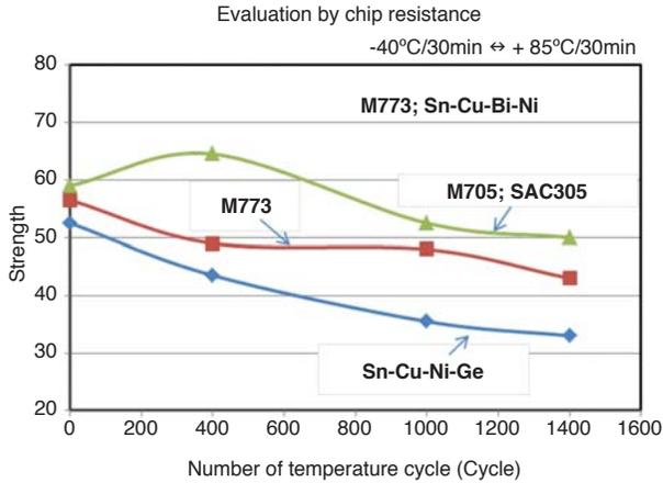
• Comparison of the progress of crack between Sn-Cu-Ni-Ge and M773
