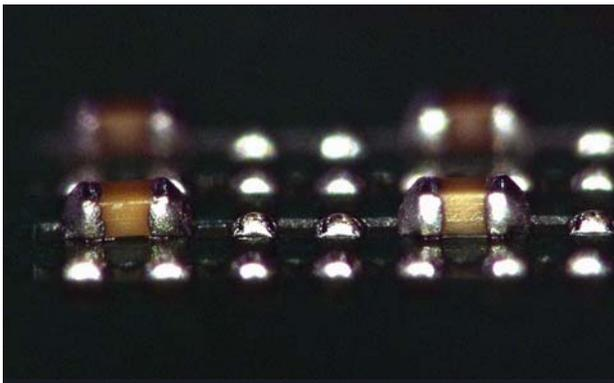
A package on which 0201 chips are mounted (Chip capacitors: Courtesy of Murata Manufacturing Co., Ltd.)
