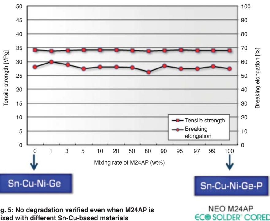
Fig. 5: No degradation verified even when M24AP is mixed with different Sn-Cu-based materials
