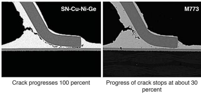
Fig. 8: Evaluation results of no-Ag solder
