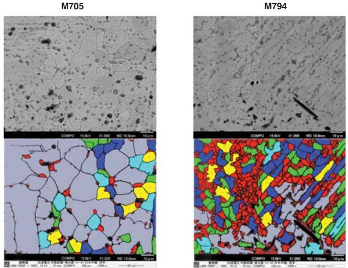
Comparison of alloy structure after 3,000 cycles
