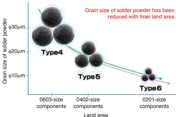
Fig. 1: Solder paste for 0201-size chip components
